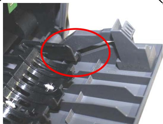
3. Pull the hook out from each side and take the back panel out
