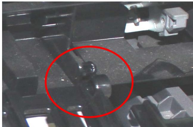
4. Pull the hook out of the inner plate on both sides.
