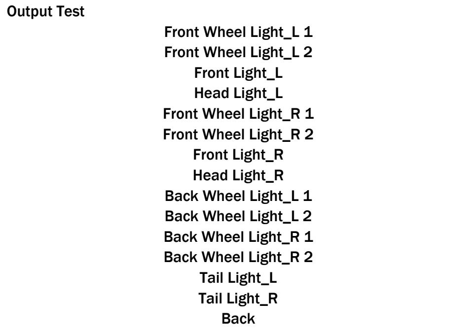
Press the Printer Reset button to select any item to be tested. Then press Volume button to confirm. When the corresponding light is on, it means the status is good.
