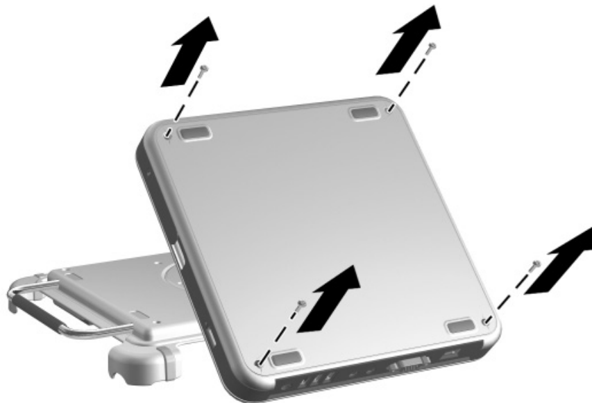
Figure 5-30. Removing the Top Case Screws
